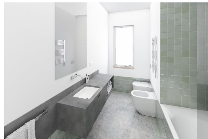
Common bathroom semi-manual tiles and painted walls concrete floor varnished Viroc cabinet (TBC) enameled bathtub Sanitana, Cifial and Bruma equipments towel warmer
